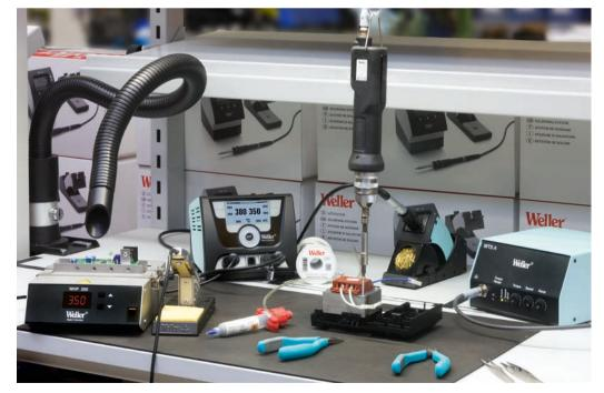
from the two 80 W and 120 W desoldering irons with the new nozzles with longer tail and standard or vertical design, to the hot air units from 100 W to 700 W. These solutions are available for connection to the compressed air network or with pump integrated in the control unit.
